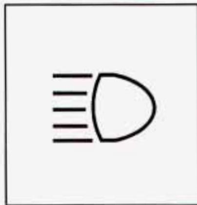
To change the headlamps from low beam to high or high to low, pull the turn signal lever all the way toward you. Then release it. When the high beams are on, a light on the instrument panel also will be on.
