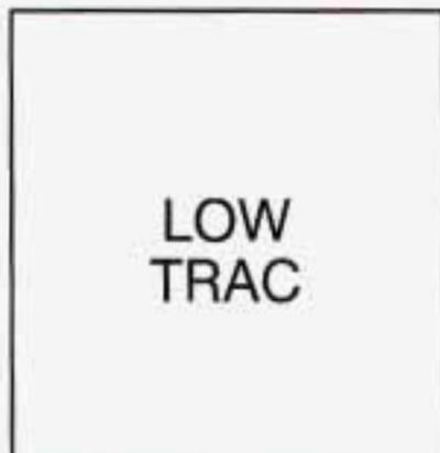
When your Enhanced Traction System is limiting wheel spin, this light will come on. Slippery road conditions may exist if the Enhanced Traction System active light comes on, so adjust your driving accordingly.
