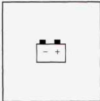
The charging system indicator light will come on briefly when you turn on the ignition, but the engine is not running. The light will go out when the engine is started.
