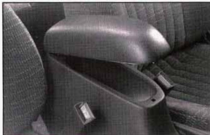
The armrest opens into a storage area for cassette tapes, gloves, etc. To open it, lift up on the front portion of the armrest.
