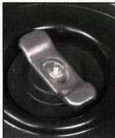
Turn the wing nut counterclockwise and remove it. Then lift off the spacer and remove the spare tire.
