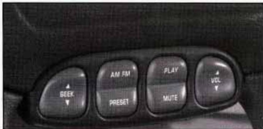
If your vehicle has this feature, you can control certain radio functions using the buttons on your steering wheel.
