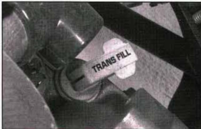
The manual transaxle dipstick is white and is located on the driver's side rear of the engine.
