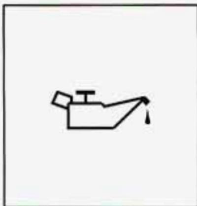
If you have a problem with your engine's oil pressure, this light may *stay on* after you start your engine, or *come on and stay on* when you are driving. This indicates that oil is not going through your engine quickly enough to keep it lubricated.
