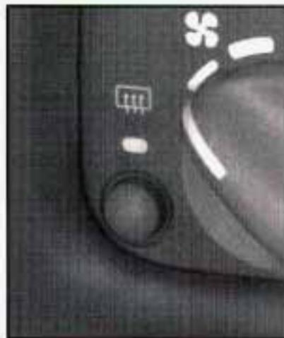
The rear window defogger uses a warming grid to remove fog from the rear window. Press the defogger switch. The indicator light will glow.
